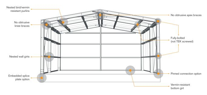
Our unique, patented Bracketless Portal System is constructed using cold-formed flat Z450 galvanised coil.
