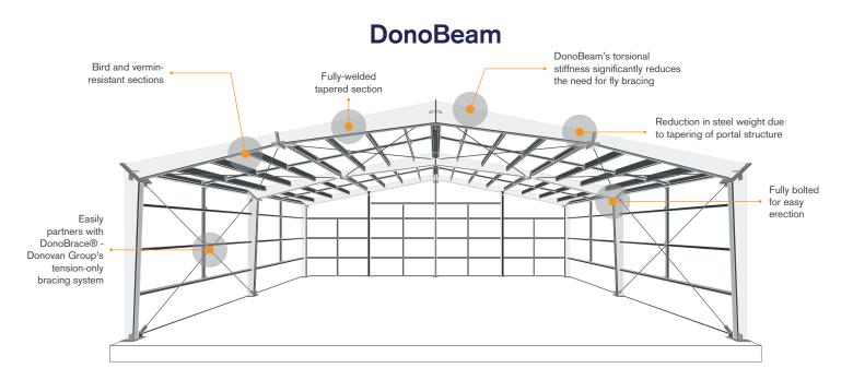
DonoBeam is manufactured by folding two halves of steel plate and welding them together to form a box. The box is tapered through its length, utilising only the amount of steel required, which reduces the weight/cost without affecting structural integrity. Using the DonoBeam system, we can achieve impressive spans suited to your business needs.
